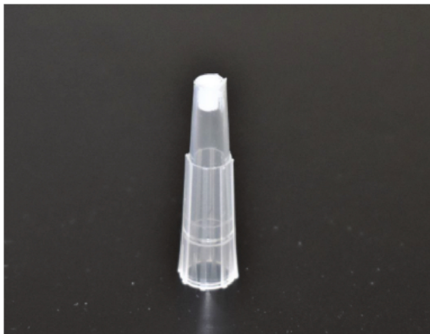
Figure 4: Plug for sealing the flow-damping enclosure. The plug can be made by sealing a 20 \mu L pipette tip with heat. Please click here to view a larger version of this figure.
